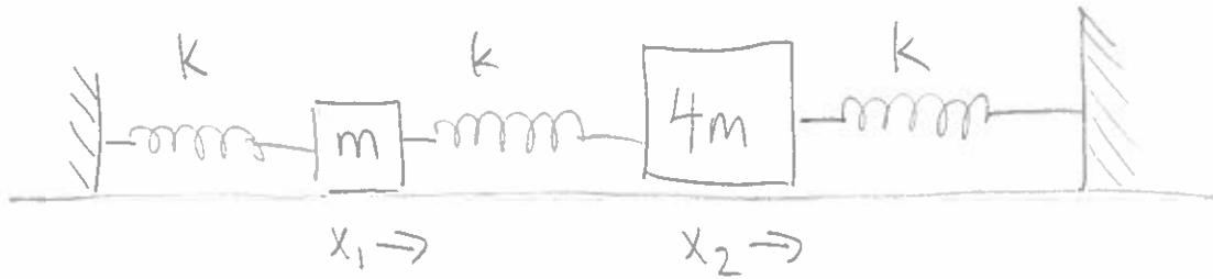
Mass  $m = 2\text{ kg}$ ,  $4m = 8\text{ kg}$  attached to springs of  $K = 24\text{ N}$ .
