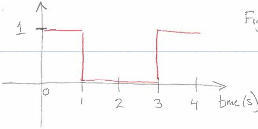
Figure at left shows one cycle of a square wave, with period  $P = 4 \text{ s}$ .
