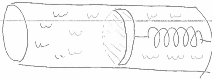
A cylinder filled with water contains a piston of mass  $m$  and spring of force constant  $k$ . The water yields a resistive force coefficient  $b$ .
