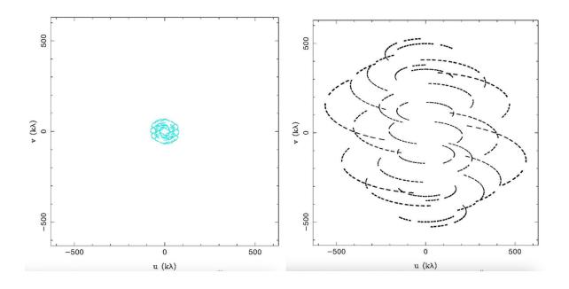
The right is the longer baseline array because of the longer u-v distances. u and v are spatial frequencies. High spatial frequencies are due to fine structure probed by long baselines.
